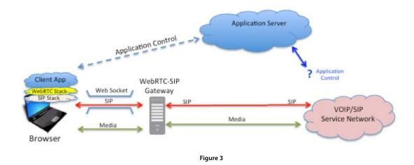
An even bigger issue that must be addressed is handling Web security issues such as CORS (Cross-origin Resource Sharing). A question for the industry now is: Where does this WebRTC-SIP gateway functionality reside? Is it a separate element that front ends the service network? Is it built into an existing element such as an SBC, media server or legacy application platform?
